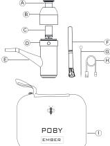
A:Infusion Cap F:Boar Brush B:Glass Cap G:Cleaning Brush C:3D Heater H:USB-C Cable D:Battery Base I:Carring Case (Different on options)
