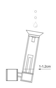
STEP 1: Screw the pearig atomizer on a 510 threaded box mod. The minimum output power of the mod is 15W.
